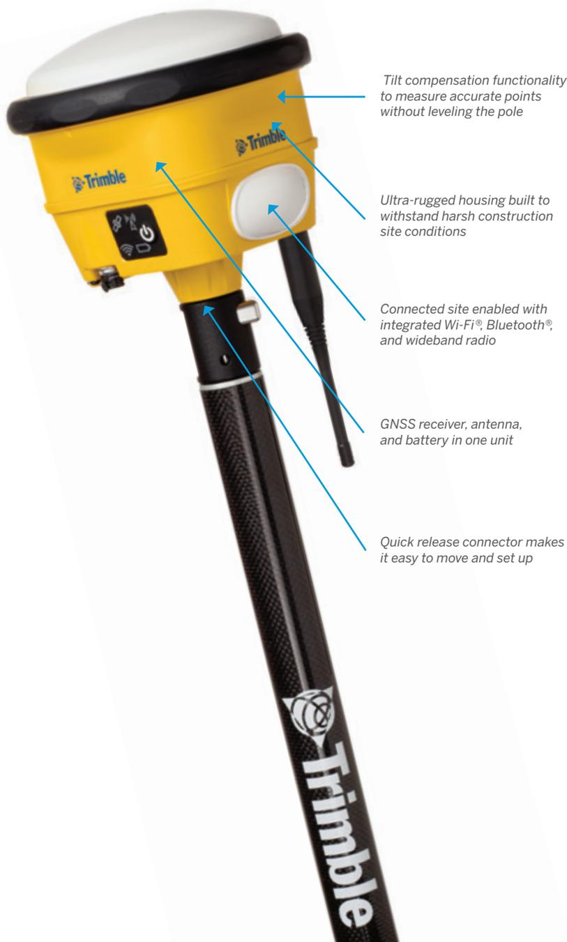
Tilt compensation functionality to measure accurate points without leveling the pole
