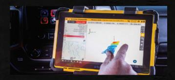
The **Trimble Siteworks Positioning System for Supervisors** includes the SPS986 or SPS785 GNSS Smart Antenna, T7 or T10 Tablet and Siteworks Software. Construction supervisors can run full office software packages and work easily with data and 3D models in the field without carrying a laptop.
